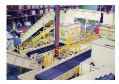
EZ-TRAX Conveyors fit many applications, such as this MRF in Lakeville, MA. It features dozens of sliderbed conveyors, sorting lines, sorting bins, platforms, and baler feed combination steel-belt conveyors.
