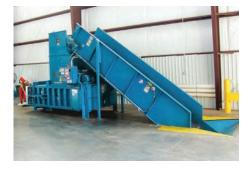
EZ-TRAX sliderbed and steel-belt conveyors are ideal add-ons for baler and compactor-feed applications. They add efficiency to optimize productivity and throughput capacity. This belowground sliderbed is feeding a Gemini® 3560 manual-tie, horizontal baler.
