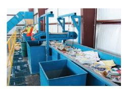
This smaller MRF, located in Bedford County, VA, has a sliderbed sorting line conveyor fed by a combination chain-belt conveyor.
