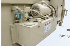
The RJ-500 and RJ-500HD come standard with the Marathon side-mounted power unit. The power unit offers the convenience and ease-of-maintenance of a remote power pack with the space savings of an integrated power unit.
